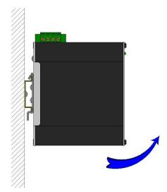
To remove the unit from the 35mm industrial DIN rail, pull forward on the unit until it disengages from the bottom of the DIN rail. Rotate the bottom of the unit towards you and up at an approximate 15° upward angle to completely remove the unit.
